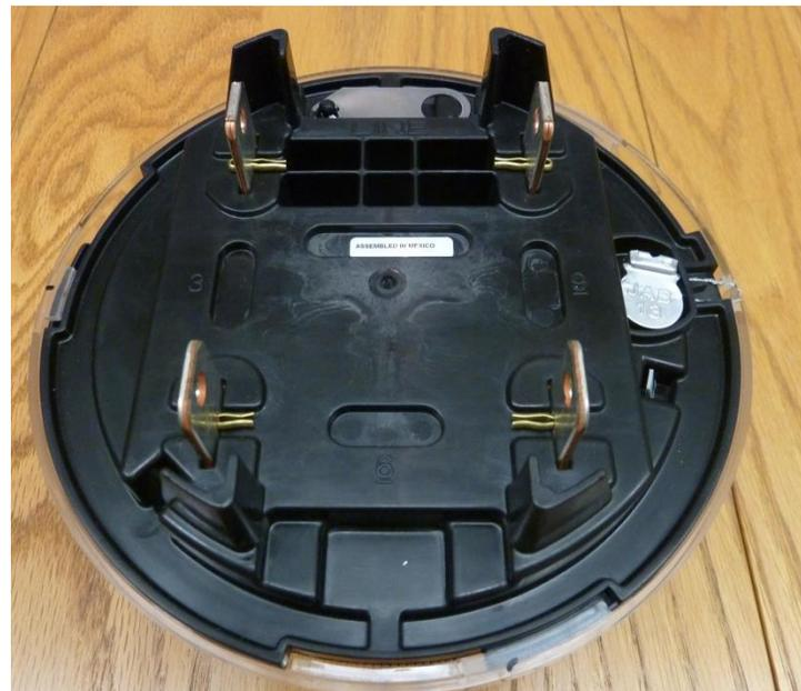
Figure 2: Back plane of assembled Sensus meter
